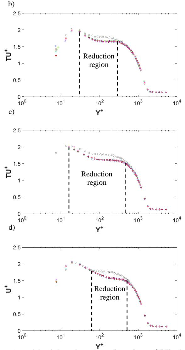
Figure 4: Turbulence intensity profile at  $Re_\theta = 3771$ . a)  $x^+ = 5.5 \times 10^3$ , b)  $x^+ = 8.2 \times 10^3$ , c)  $x^+ = 10.9 \times 10^3$ , d)  $x^+ = 13.9 \times 10^3$ . (o) No control, ( $\Delta$ ) cavity array – No excitation, (+) 500Hz excitation, ( $\square$ ) 1000Hz excitation, ( $\diamond$ ) 2000Hz excitation, (x) 4000Hz excitation, (\*) 8000Hz excitation
