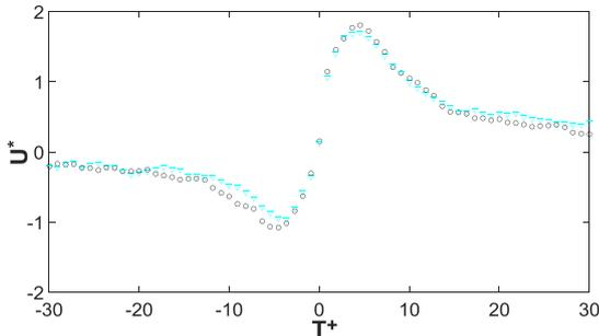
Figure 5: Average VITA sweep events at  $Re_\theta = 3771$ ,  $x^+ = 10.9 \times 10^3$ . (o) No control, ( $\Delta$ ) cavity array – No excitation
