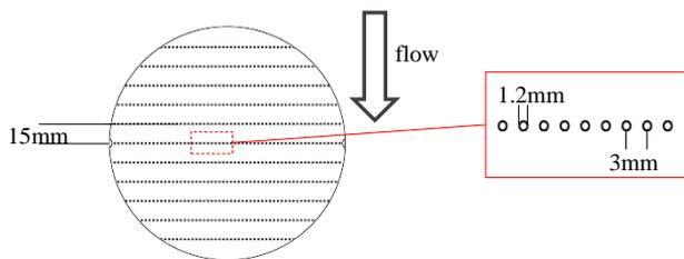
Figure 2: Schematic of the cavity array
