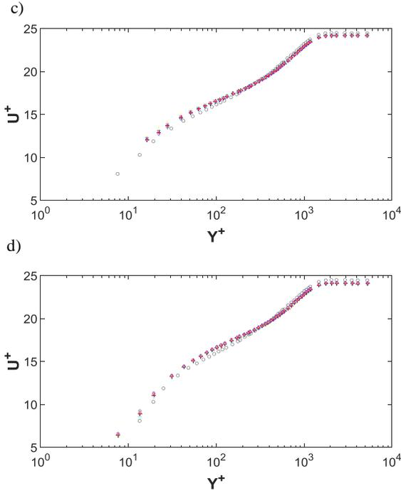
Figure 3: Mean velocity profile at  $Re_\theta = 3771$ . a)  $x^+ = 5.5 \times 10^3$ , b)  $x^+ = 8.2 \times 10^3$ , c)  $x^+ = 10.9 \times 10^3$ , d)  $x^+ = 13.9 \times 10^3$ . (o) No control, ( $\Delta$ ) cavity array – No excitation, (+) 500Hz excitation, ( $\square$ ) 1000Hz excitation, ( $\diamond$ ) 2000Hz excitation, (x) 4000Hz excitation, (\*) 8000Hz excitation
